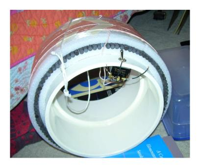
In order to lower the FSL into the enclosure, the FSL must be first partially lowered in to clear the variable capacitors. Once the capacitors and the switch are close enough together, the connections can be made, and the FSL can be lowered all the way in. <u>This can be tricky</u> – you might want to have someone holding onto the FSL while you make the connections!
