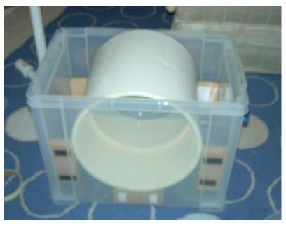
The next step was to wrap one layer of half-inch thick foam around the coupler, providing a foundation for the ferrites. Note that the foam stops about one inch from the edges of the PVC coupler in order to provide a place for the supporting blocks to contact the PVC coupler.
