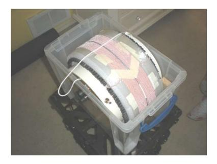
To use the finished FSL, simply select which band you want using the DPDT, and tune the antenna to the resonant frequency. I purposely put the band switch inside in order to make the FSL more weather-resistant (and to allow the PVC to fit inside the box), and it is a simple matter of momentarily lifting the lid to switch bands.
